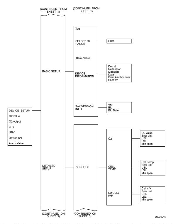
Figure 4-3. Menu Tree for HART/AMS on the Two-Wire In Situ Oxygen Analyzer (Sheet 2 of 3)
